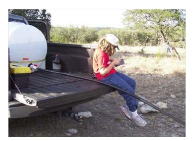
Initially we used a 250 gallon tank on the truck but that much water weighed over a ton and bent the axle of the truck. Over time we found the average usage at this rain catcher was about 50 gallons/week except during the driest parts of the summer when it went to 100 gallons/week.
